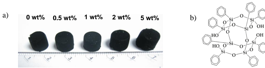
Figure 1: (a) Photographs of as-prepared 3D-graphene aerogels with different content of tetra-POSS; b) Chemical structure of Tetra-POSS
